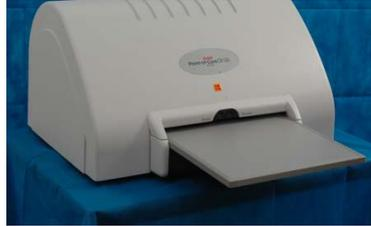
Fig. 2 - An example of a cassette reader used in CR
